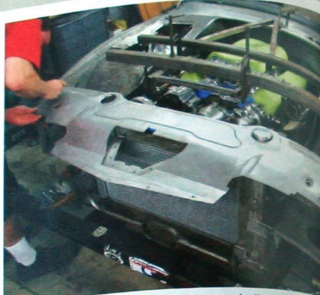
> In this under-construction shot you can see the jig setup that's use to hang the turbos and to aid in the fabrication of all the bracketry and to hang the turbos. The entire nose of the car was also reworked accept the Ron Davis intercooler and radiator as well as the air dum
