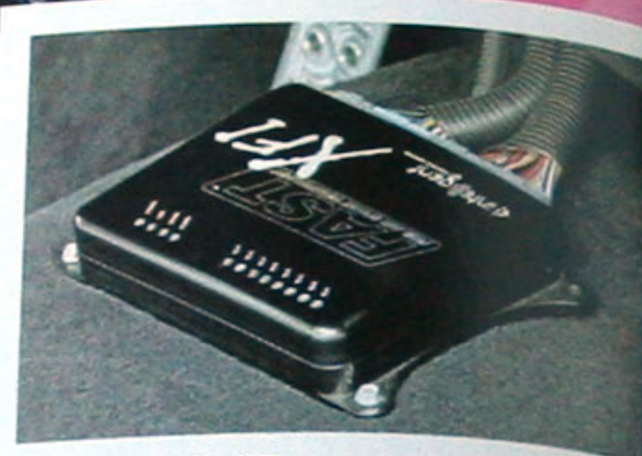
FAST Man EFI's XFI computer adds traction control and engine management to Ed's Challenger.
