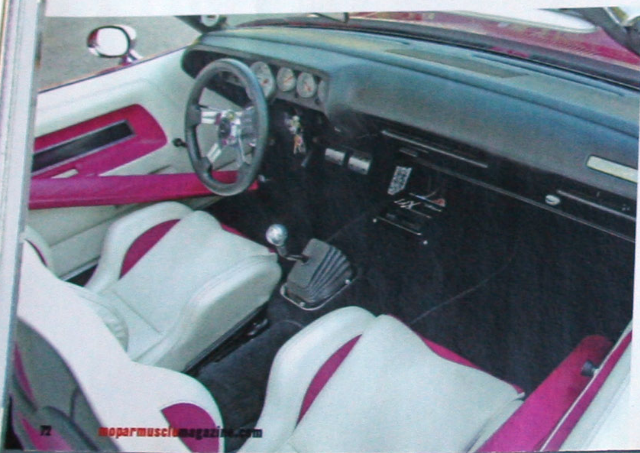
Gauges, Tremec shifter, and a FAST XFI computer from FAST Man EFI are joined by custom Cobra buckets and a Grant GT wheel. Cobra buckets and four-point rollbar add function to the Challenger's interior, though the bar might not meet LVMS rules if Ed turns 11.00 seconds or better in the quarter-mile.
