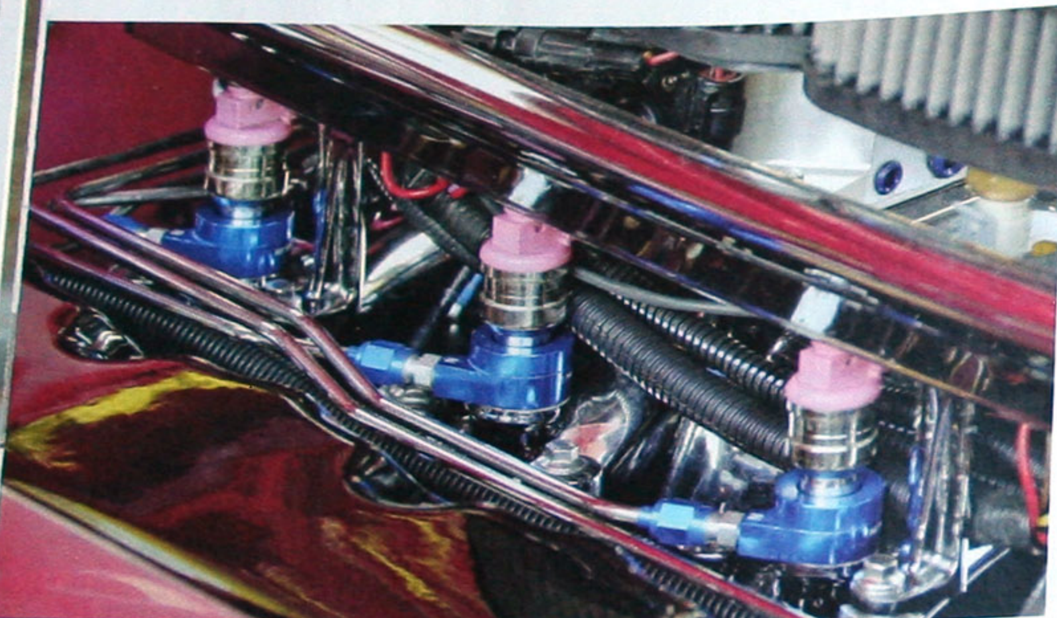
Blue nozzles under each injector are Holley Race NOSzles, supplying each fuel injector with enough go-go gas to bump the Hemi's output from 700 hp to around 830 hp.
