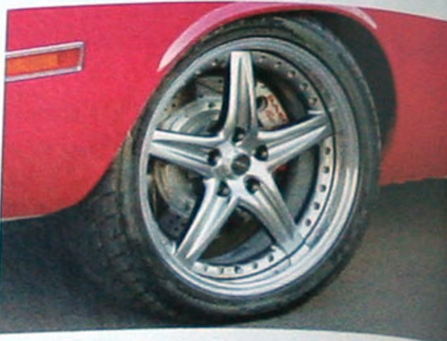
Multi-piece ROH wheels wear low-profile Nitto tires while fronting big Baer disc brakes.
