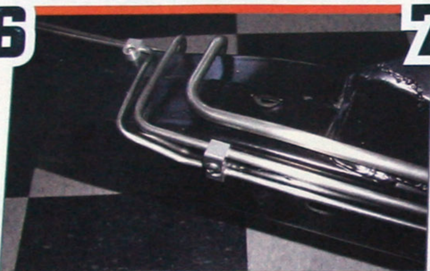
All three metal lines run parallel—even during bends. Notice the custom brackets.
