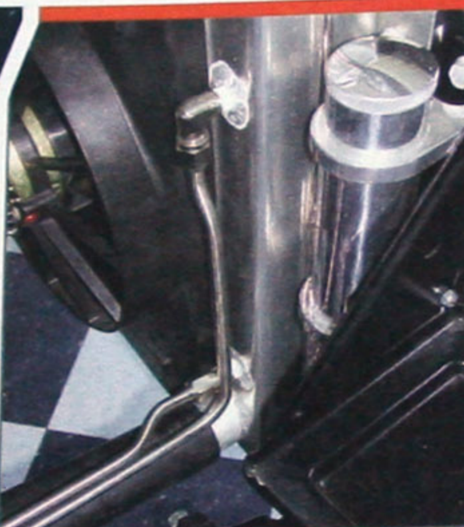
Gannon's automatic transmission has to/from Bent Fabrication metal lines attached to the radiator-side cooling tank. Note that everything is expertly positioned and exact.
