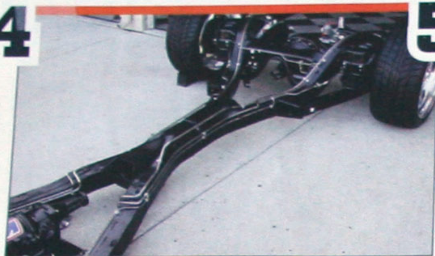
This photo of Bill Gannon's '61 "X" frame fully dramatizes Bent Custom and Performance's brake, fuel and airbag lines. We feel your mental gears starting to roll.
