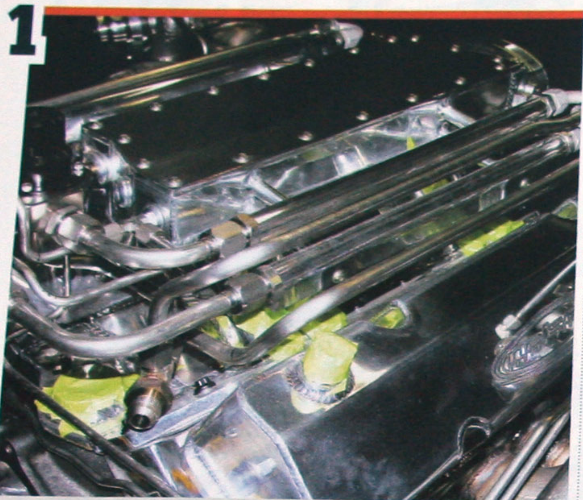
All the lines you see on this Tom Nelson racing engine were Mark Bohlen-built from scratch. Regular metal lines do not have the molecular structure for polishing. Stainless steel lines do, and they have the added benefit of retaining a shine.
